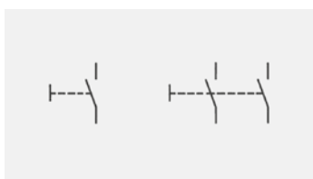
Normally open contact (momentary) / pushbutton (SPNO, DPNO)
