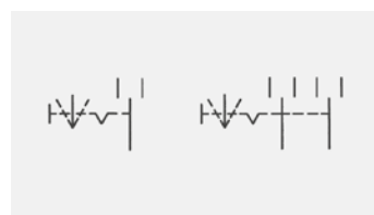
Changeover switch with OFF position in the center (SPDT-Center OFF, DPDT-Center OFF)
