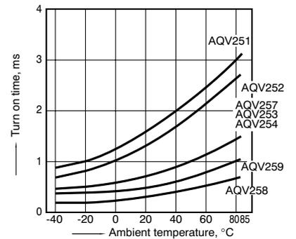
3.-(2) Turn on time vs. ambient temperature characteristics
