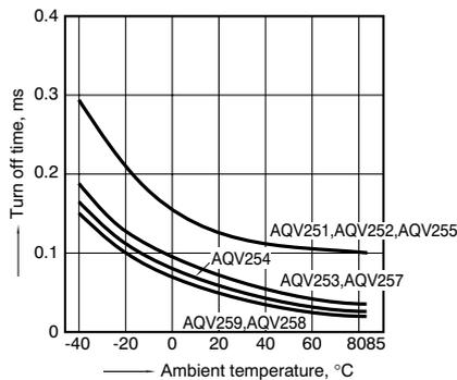
4.-(2) Turn off time vs. ambient temperature characteristics
