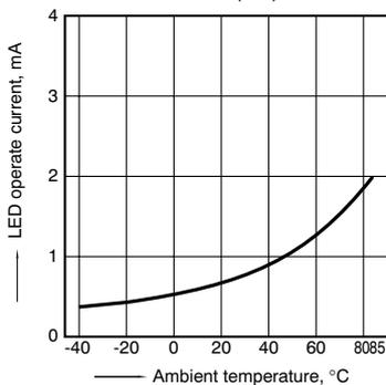
5.-(2) LED operate current vs. ambient temperature characteristics
