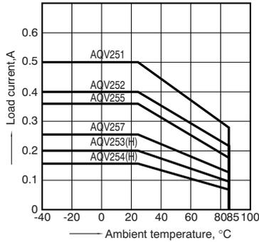
1.-(2) Load current vs. ambient temperature characteristics
