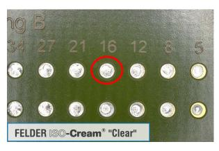
As this example shows the paste has excellent wetting qualities in comparison to a conventional solder paste (here on Ni/Au). Even with low solder paste application (here 16 % of the pad area) a 100 % wetting of the solder surface is reached.
