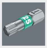
BTZ-Bits have an additional tempered BiTorsion zone, which reduces the hardness of the shaft by about 20 % in comparison to the drive tip. This means that the peak loads that cause bit breakage and premature wear are absorbed in this zone — something which enhances the service life of the bits.
