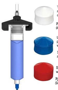
The tighter fit wiper pistons are recommended for use with low viscosity fluids and mechanical devices, such as a manual syringe gun, to prevent leakage past the double wiping edges
