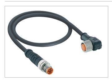
M8 actuator/sensor cordset with overmolded connectors, with self-locking threaded joint, IP 67
