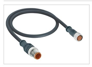
M12/M8 actuator/sensor cordset with overmolded connectors, with self-locking threaded joint, IP 67
