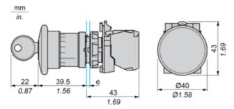
e: clamping thickness: 1 to 6 mm / 0.04 to 0.24 in.
