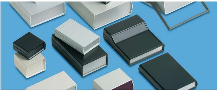
The FRONT PANEL series, available in over fifty models, is ideally suited to a variety of electronic desktop applications. The enclosures are manufactured from high ABS or high impact polystyrene. They are available with either aluminium or plastic front and rear panels. All models have internal guide and PCB mounting studs.
