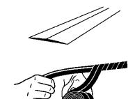
The use is simple. The rolling up of the layers must be done by overlapping the preceding one of half. The triangular shape of the ribbon makes it possible to obtain a regular thickness thus.
