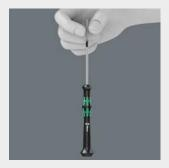
The electronic TORX® screwdriver with holding function (HF) literally presses the screw onto the screwdriver. The conical driving flanks that taper toward the tip of the tool, the optimised flank base and the ideal engage depth hold the screw securely on the blade.
